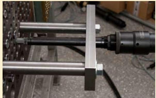
Mock up of Fin Fan cooler 10" long water box and 1" tubes
